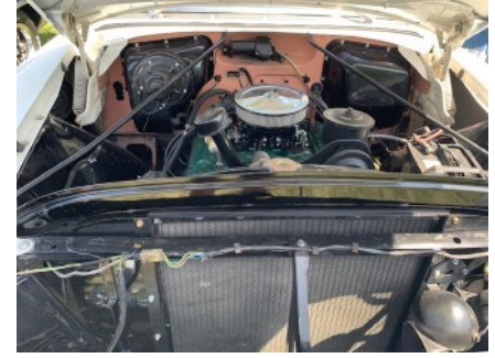
Rocket 88 power! 324 ci, originally 230 HP with 340 ft/lbs torque, upgraded w/Edelbrock fuel delivery.
