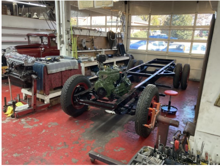
Chassis of the M16 Studebaker truck. Cab in Metal Shop getting work.
